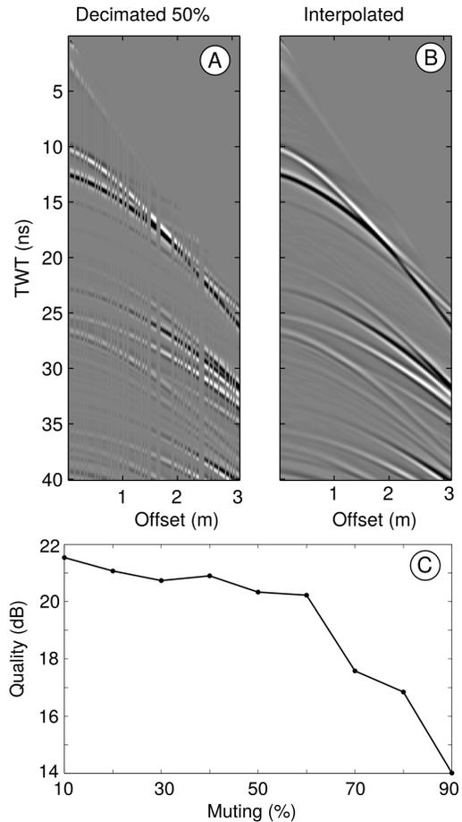
Figure 2: Model experiments. In **A** model with 50% of null traces, **B** Reconstruction and **C** a graph showing quality of reconstruction versus decimation factor.
