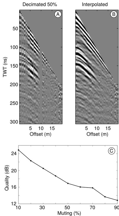
Figure 3: Real Data. In **A** model with 50% missing data, **B** reconstruction results and **C** a graph showing the quality of reconstruction versus decimation.
